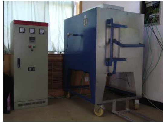
Fig. 1. Box heating furnace.
