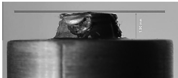
Fig. 2. Appearance of the torn tool after being pushed into steel sheet during FSW operation.
