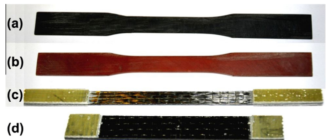
Fig. 1. (a) MWCNTs/epoxy, (b) Neat epoxy, (c) longitudinal MWCNTs/CF/epoxy and (d) transverse MWCNTs/CF/epoxy specimens prepared for the tensile test.
