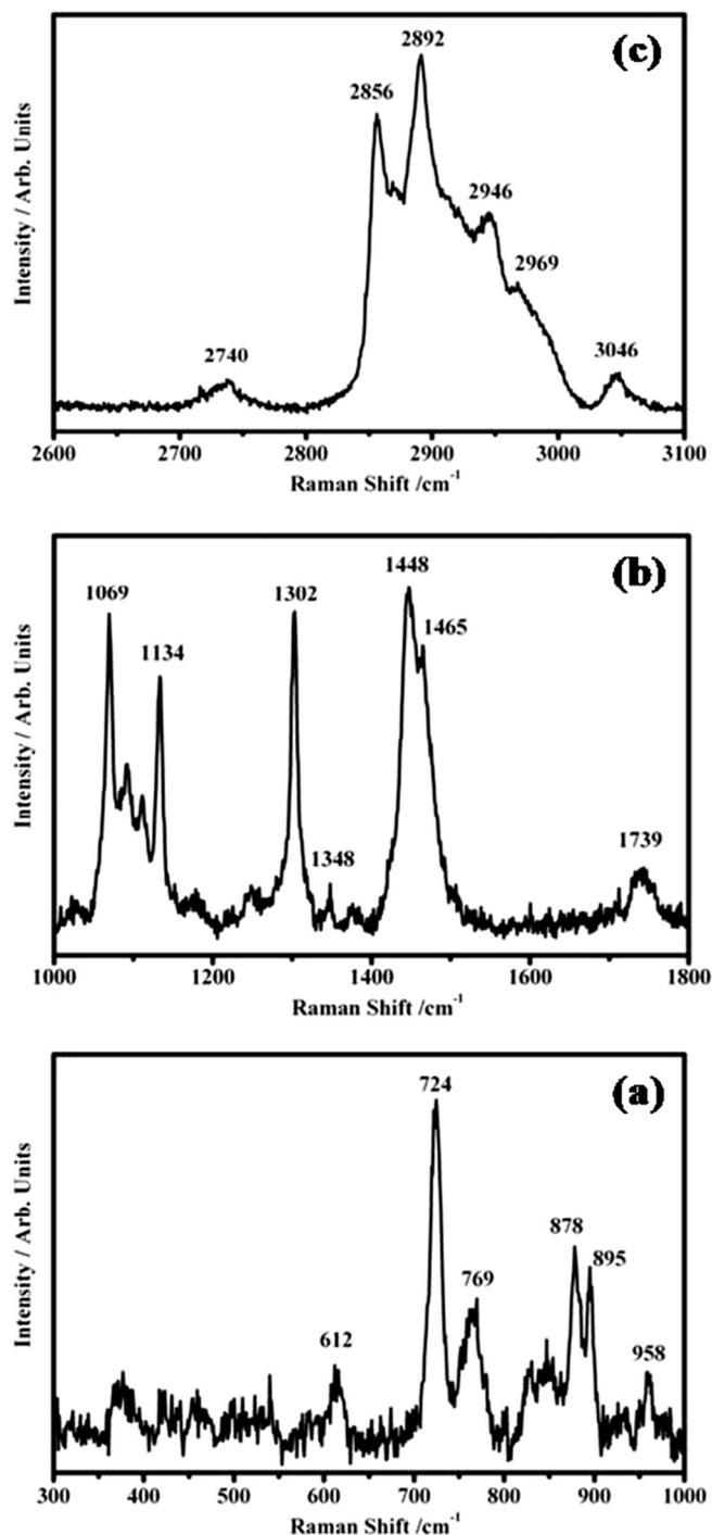
Fig. 1. Representative Raman spectra collected on the 1,2-dimyristoyl-sn-glycero-3-phosphocholine (DMPC) powder in the range between 300 and 1000  $\text{cm}^{-1}$  (a), 1000 and 1800  $\text{cm}^{-1}$  (b) and 2600 and 3100  $\text{cm}^{-1}$  (c).
