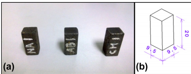
Fig. 1. (a) Prepared frictional brake pad specimens and (b) specimen dimensions.
