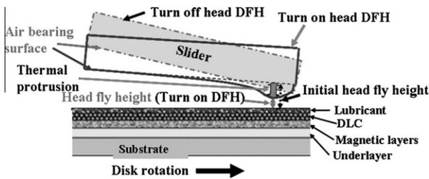
**Fig. 1.** Schematic of head disk design interface with a thermal protrusion slider (illustrates the head fly height was reduced from 10 down to 1.5 nm after turn on head DFH).
