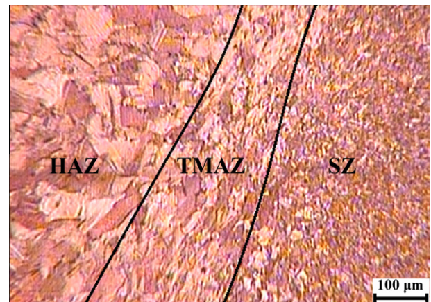
Fig. 3. Microstructure of sample welded by threaded cylindrical pin profile showing the SZ, TMAZ and HAZ (rotation rate of 600 rpm and traverse speed of 75 mm/min).
