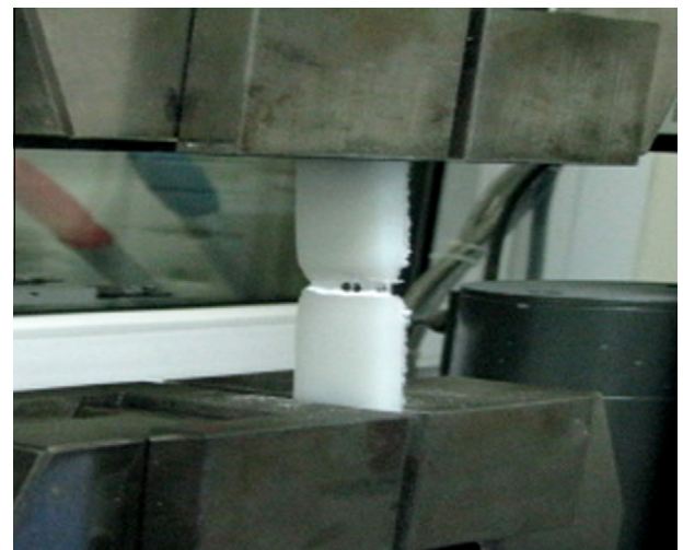
Fig. 2. Tensile test operation of the HDPE sheets joined by FSW.
