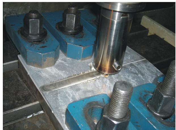
Fig. 2. Friction stir welding process.
