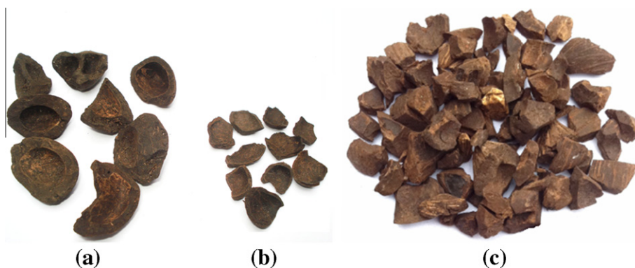
Fig. 1. OPS aggregates: (a) original large size, (b) original small size, and (c) crushed from original large size.
