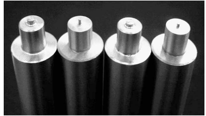
Fig. 2. CDW specimens with different igniter dimensions.
