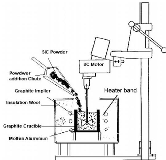
Fig. 1. Schematic of the stir casting set-up used for the fabrication of Al/SiC<sub>p</sub> composite.
