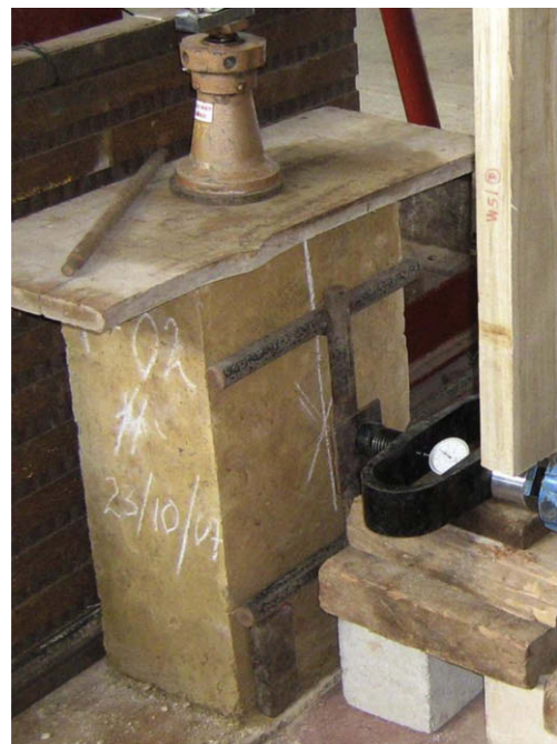
Fig. 5. Rammed earth panel of 600 mm of length × 900 mm of height × 150 mm of thickness used for testing.
