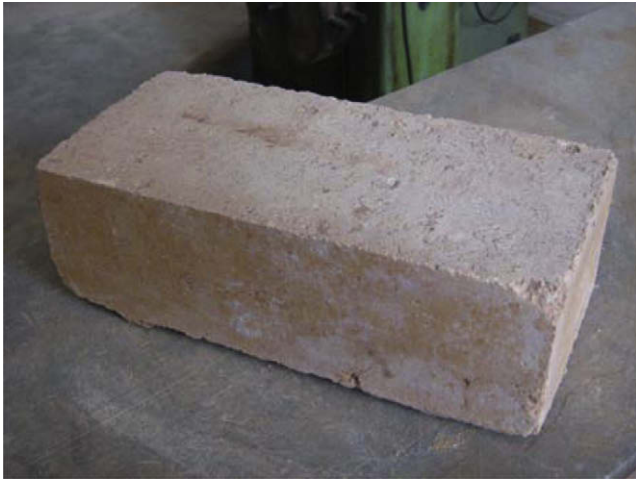
Fig. 1. CSE brick of 230 mm × 110 mm × 75 mm (length × width × height).
