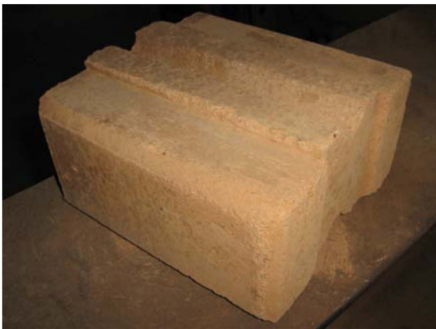
Fig. 3. CSE interlocking solid block of 225 mm × 225 mm × 115 mm (length × width × height).
