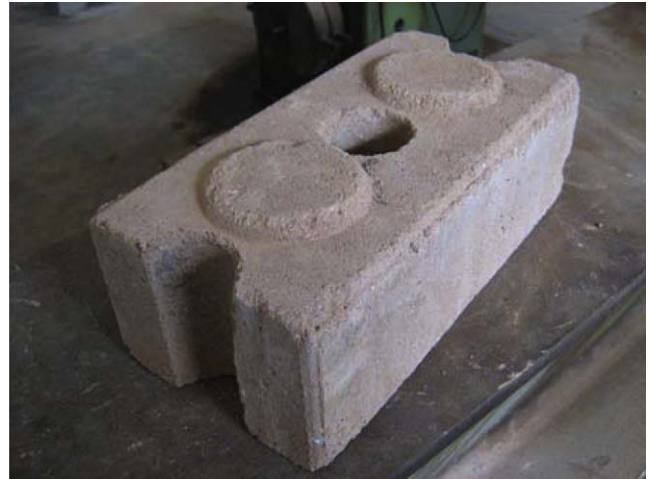
Fig. 4. CSE interlocking hollow block of 300 mm × 145 mm × 100 mm (length × width × height).
