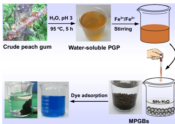
Fig. 1. Schematic illustration of the preparation of magnetic peach gum beads (MPGBs) from crude peach gum for dye adsorption.
