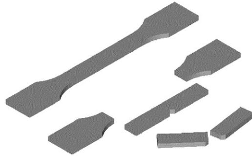
Fig. 1. Cold drawn impact samples manufacturing procedure.
