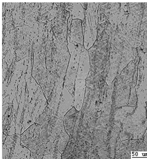
Fig. 2. Optical micrograph of TiNi alloy before the first ECAE process.
