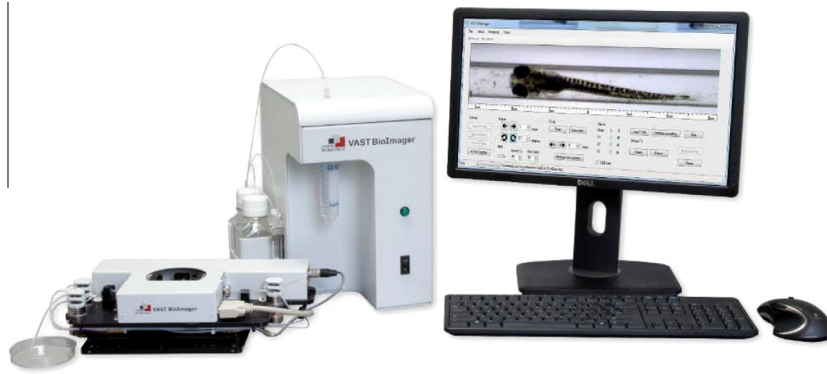
Fig. 1. VAST BioImager is composed of two parts, the imaging unit (left) and the controller unit (center). A computer/monitor runs the software that controls the VAST BioImager and collects the larval images.
