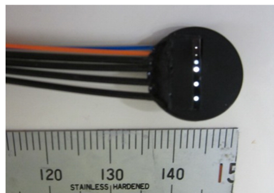
Fig. 1. Sensor probe (o.d. 10 mm). Six optical fibers are incorporated in a line at the center of the probe: (1) used to detect light for laser Doppler blood flow measurement; (2) used to produce light for laser Doppler blood flow measurement; (3) used to produce light for tissue blood oxygenation measurement; and (4–6) used to detect light for tissue blood oxygenation measurement.
