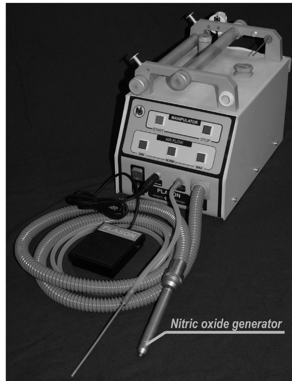
Fig. 1. Plason device for NO therapy of Center BMSTU.
