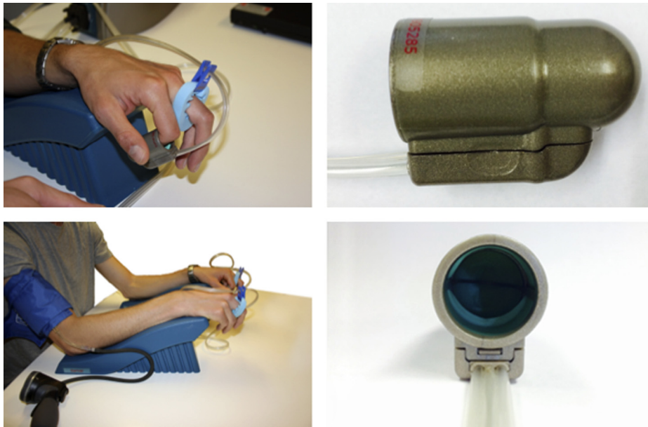
Fig. 1. (Top left) Examination settings; finger probes are placed on the index finger of each hand. A foam rubber ring disperses the index finger and middle finger, allowing the probe not to be touched which otherwise can result in artefacts. (Bottom left) A cuff is placed on the forearm and is inflated to induce reactive hyperaemia. (Top right and bottom right) The examination probe consists of a stiff external covering containing the electronically controlled inflatable chambers.
