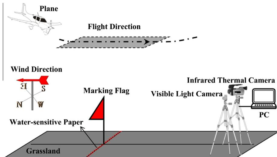
Fig. 1. Schematic diagram for monitoring of aerial spray application in the test field of Beidahuang General Aviation Company.
