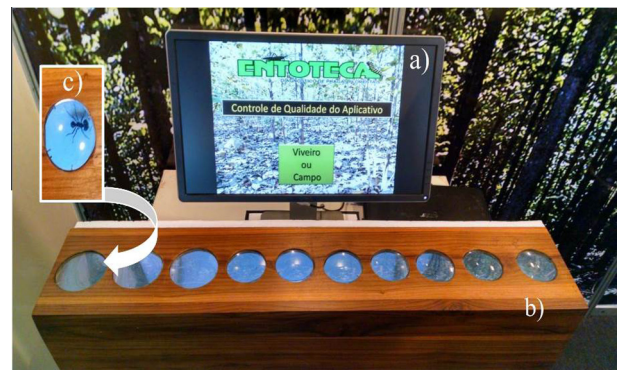
Fig. 1. (a) Device developed to validate the sensory analysis; (b) insects view to be identified; (c) magnifier.
