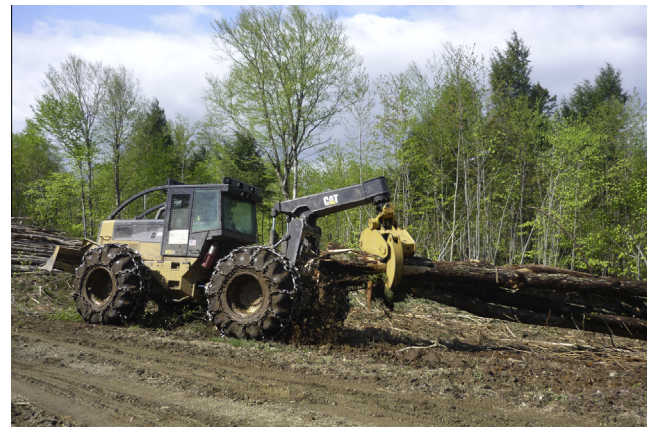
Fig. 2. A grapple skidder generally transports several trees in a bunch from the forest to the roadside where the whole trees get processed by a stroke delimeter.
