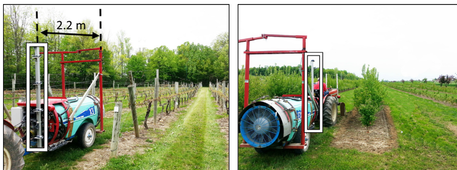
Fig. 2. Modified sprayer and sensors distribution, right orchards and left vineyards. The ultrasound are highlighted by a white rectangle.
