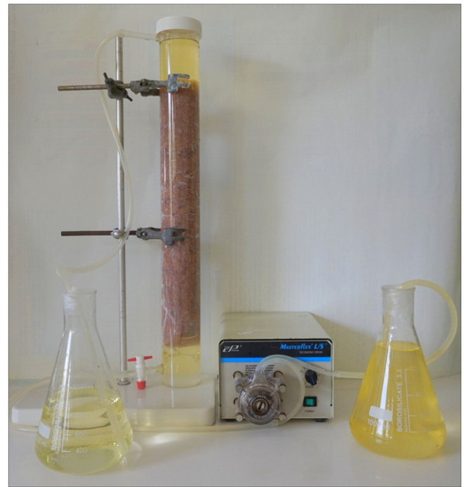
Fig. 1. Experimental set-up using a packed-bed bioreactor with tubular cellulose.
