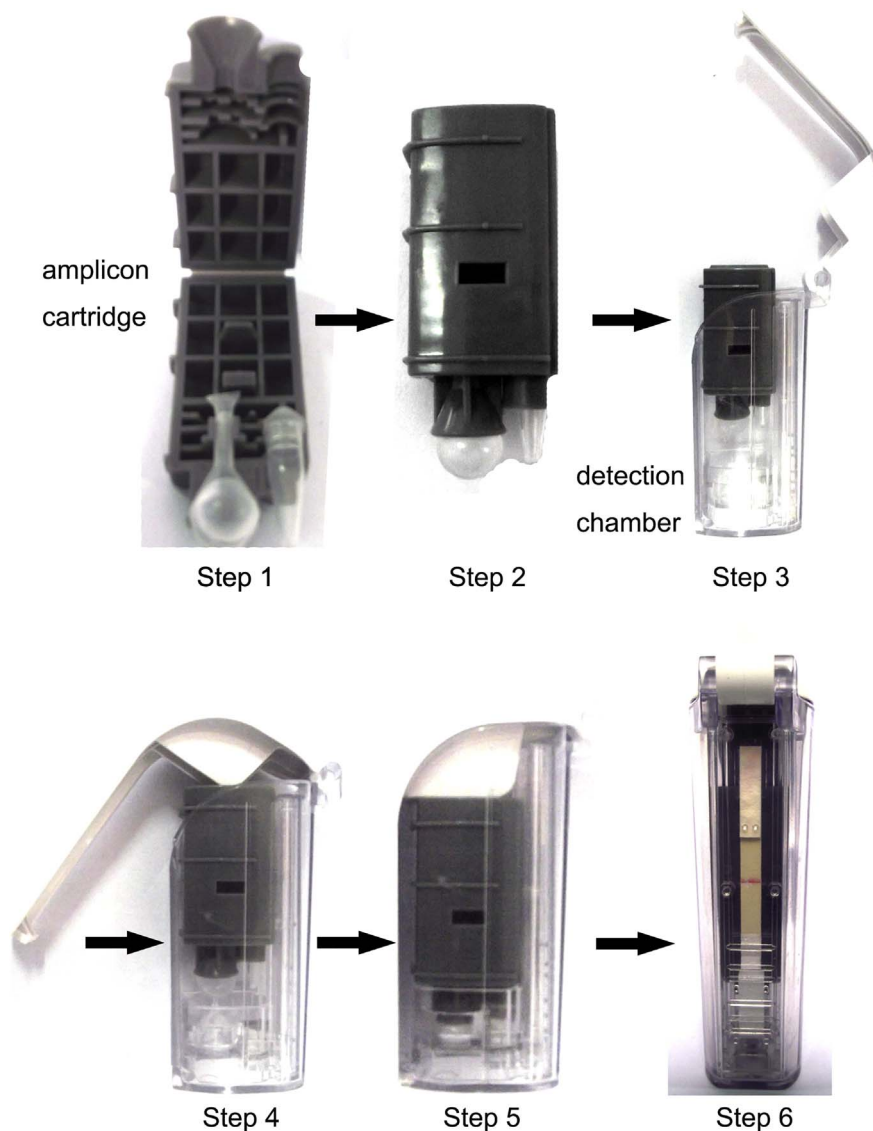
Fig. 1. The procedure of manipulating a VF visualization strip cassette. The reaction tube is immobilized in the cartridge (step 1), the cartridge is closed (step 2), the cartridge is inserted into the detection chamber (step 3), the handle of the detection chamber is pressed (step 4), the chamber is sealed, the running buffer bulb and the reaction tube are punctured simultaneously (step 5), and the results was judged visually through the detection window of the chamber after 5 min (step 6).
