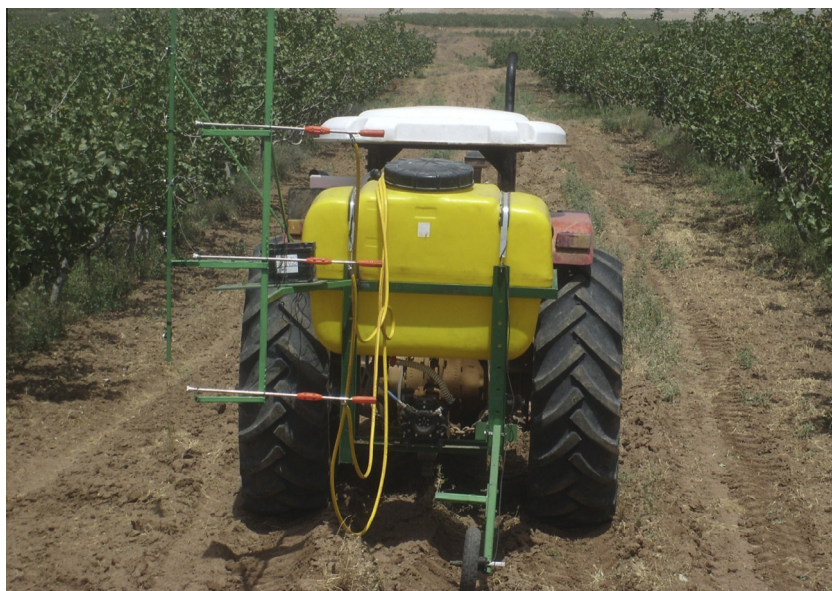
Fig. 1. Variable rate sprayer for fruit tree protection.
