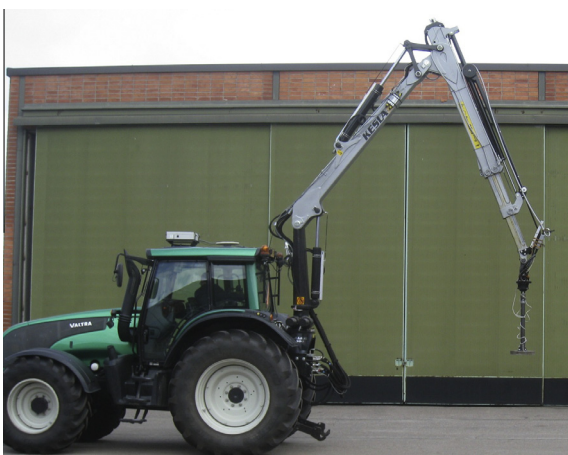
Fig. 1. Test platform consisting of an agricultural tractor and instrumented forestry crane. A freely hanging arm with a mass at the end is attached to the tip of the boom to simulate a tool.
