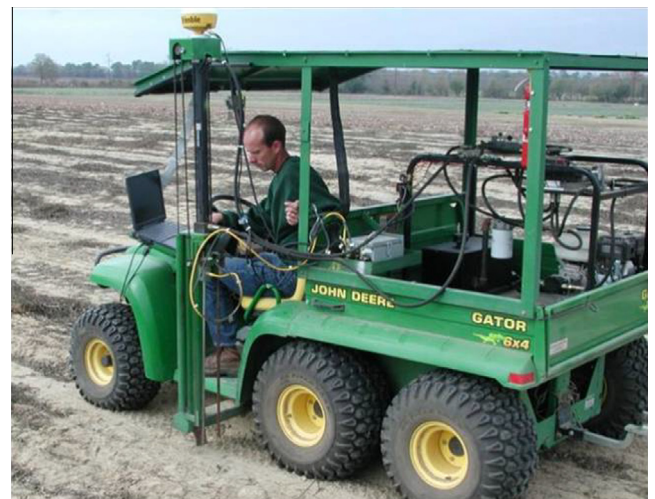
Fig. 2. Hydraulically operated, penetrometer system with DGPS unit.
