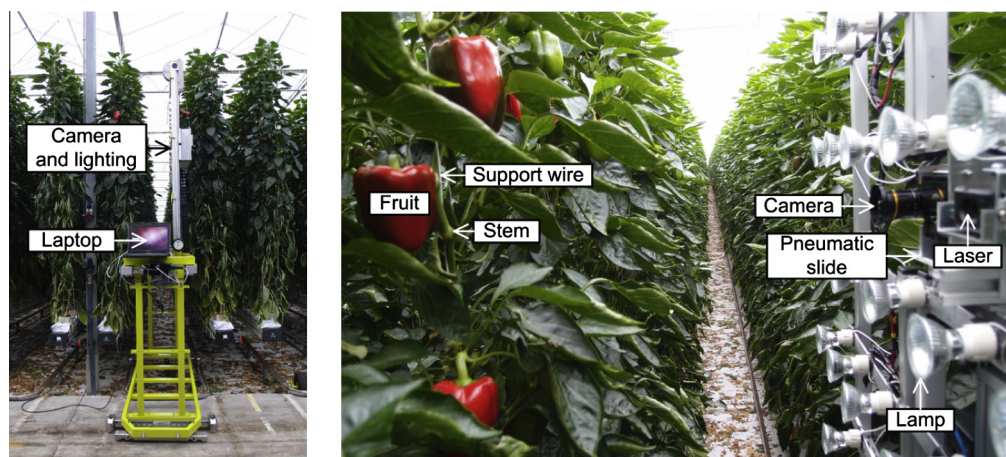
Fig. 1. Experimental set-up comprising a cart with a height-adjustable imaging set-up on top (left). Detailed view of the imaging set-up during recording in a row (right).
