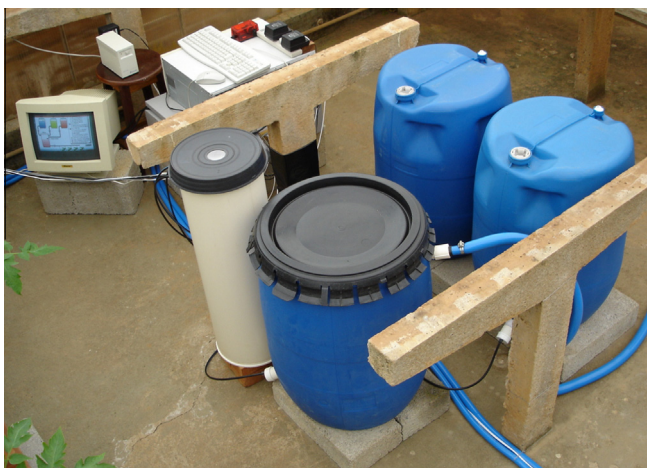
Fig. 1. Perspective view of reservoirs (mixing, stock solutions and water) and computer of the FACS.
