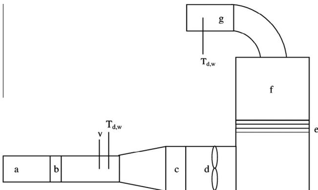
Fig. 1. Schematic diagram of test apparatus: (a) inlet duct, (b) flow straightener, (c) butterfly valve, (d) in-line duct fan, (e) perforated plates, (f) test column, and (g) outlet duct.
