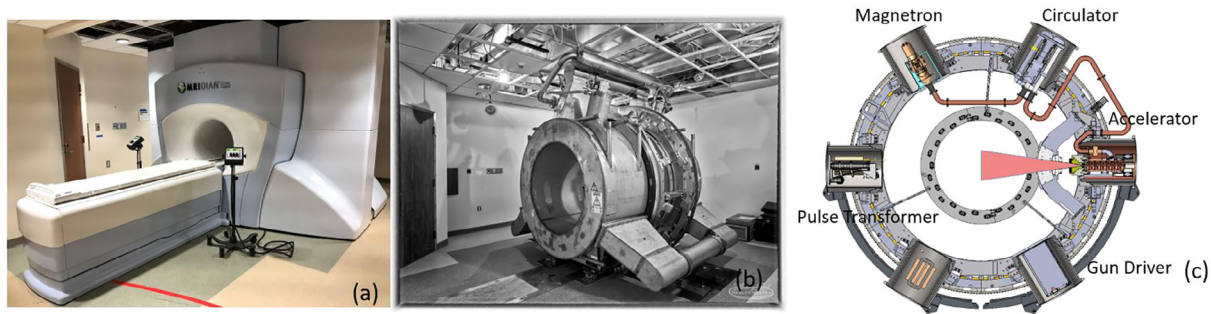
Fig. 1. (a) The MR-Linac system includes a split magnet MRI system, a rotating gantry assembly, and a patient-positioning couch with two in-room couch control panels; (b) a double-donut superconducting wide bore magnet with 0.345 T field strength; (c) the schematic of the Linac components housed in cylindrical ferromagnetic shields.
