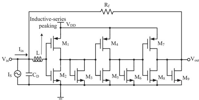
Fig. 3. Three-stage cascade push-pull inverter with inductive-series peaking.
