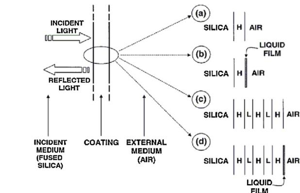
Fig. 2. Schematics of four broadband coating structures that used in simulation [8].
