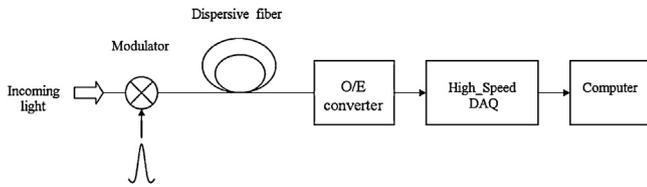
Fig. 1. Schematics of operational principle of the HSFOS [6].
