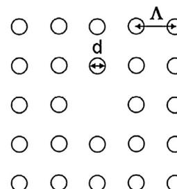
Fig. 4. Cross section of the square-lattice PCF used in the fiber optic spectrometer [12].
