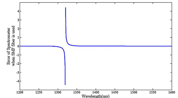
Fig. 3. The error of broadband spectrometry when SMF is used as dispersive fiber in HSFOS.
