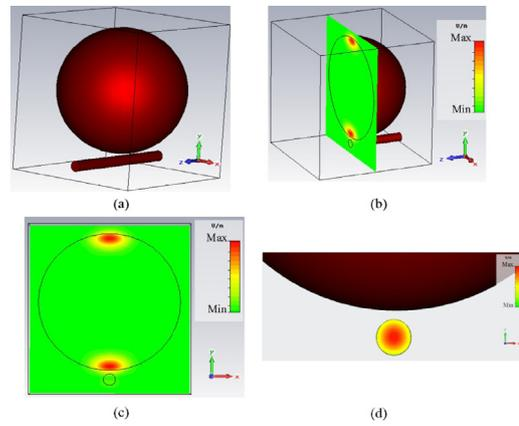
**Fig. 2.** (a) Perspective of microsphere and optical fiber system. (b) Perspective of fundamental mode of microsphere in  $x$ - $y$  plane. (c) Fundamental mode of microsphere. (d) Fundamental mode of optical fiber.
