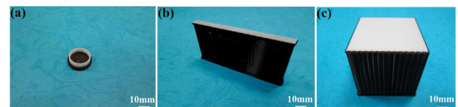
Fig. 5. Three test parts with the support structure. The white part and black part of the fused deposition molded parts indicate the modeling material and the support material, respectively.
