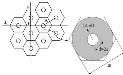
**Fig. 1.** The photonic crystal fiber cladding structure, corresponding hexagonal and circular unit cells. The straight lines  $S_1$  and  $S_2$  represent planes of symmetry of the structure.
