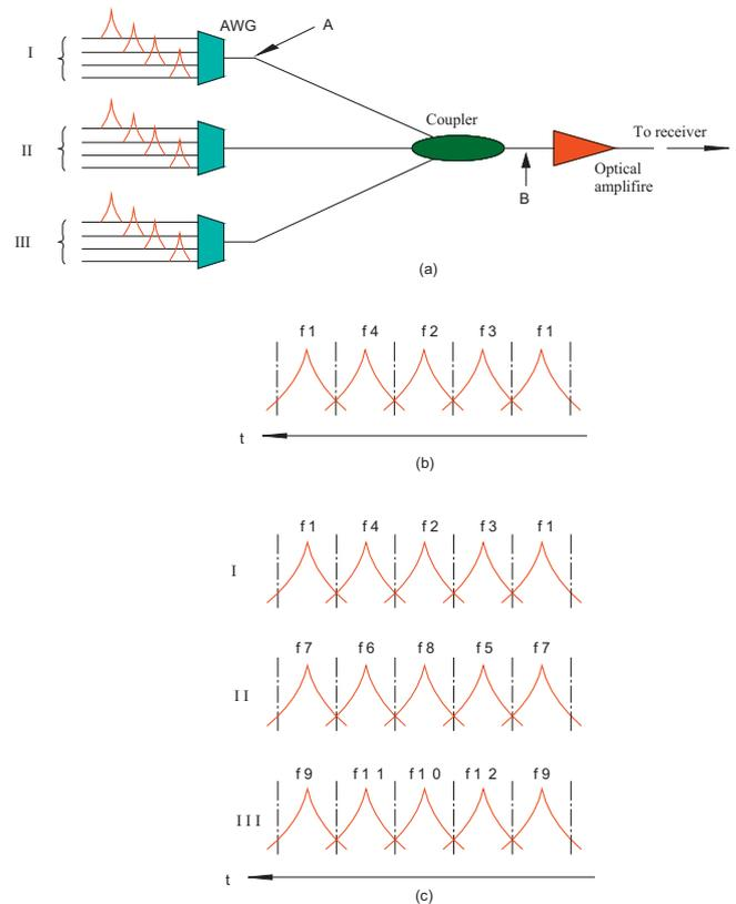
**Fig. 1.** Schematic diagrams for (a) hybrid WDM/TDM system, (b) channel arrangement at point A, and (c) channel arrangement at point B [6].
