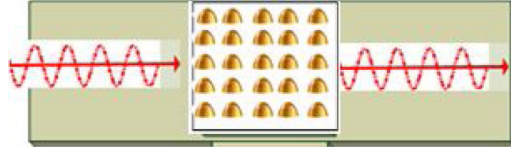
Fig. 1. Concept of plasmonic sensor by plasmonic nano bi-domes on top of SiO 2 waveguides.
