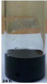
Fig. 1. Freshly prepared MWCNTs dispersed in DMF solution.
