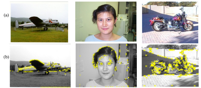
Fig. 2. (a) Sample images from Caltech database, (b) most prominent salient points detected.
