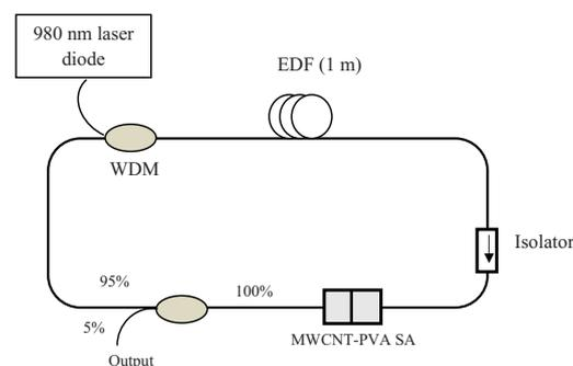
Fig. 2. Schematic configuration of the Q-switched EDFL.
