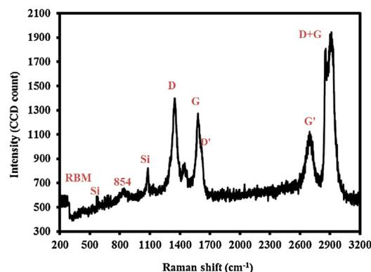
Fig. 1. Raman spectrum obtained from the MWCNT-PVA film.
