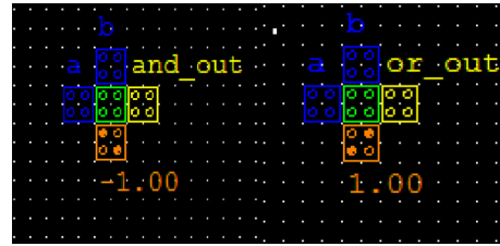
Fig. 6. Layouts of AND gate and OR gate.
