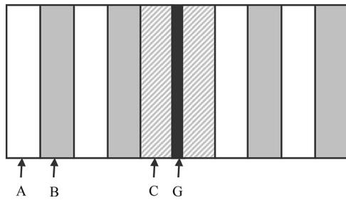
Fig. 1. Schematic of a 1DPC structure with a monolayer graphene defect layer.
