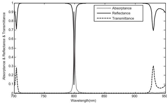
Fig. 2. Absorbance (dotted line), reflectance (full line) and transmittance (imaginary line) of 1DPC with a monolayer graphene defect at normal angle.
