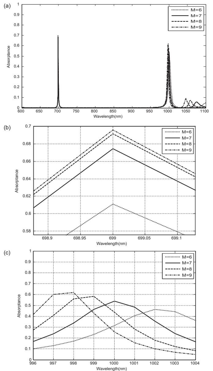
Fig. 3. (a) Absorbance as a function of wavelength for different period numbers. (b) At 699 nm, absorbance as a function of wavelength for different period numbers. (c) Around 1000 nm, absorbance as a function of wavelength for different period numbers.
