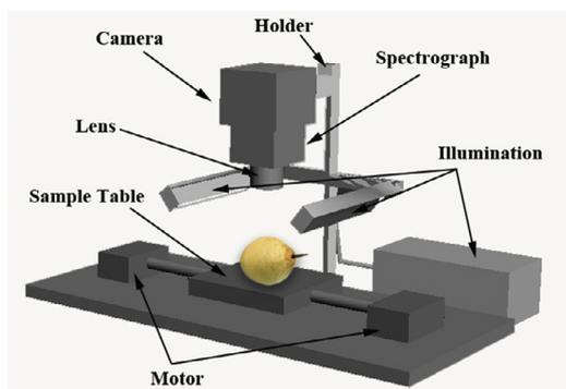
Fig. 1. Schematic diagram of the main components of the imaging spectrometry system.
