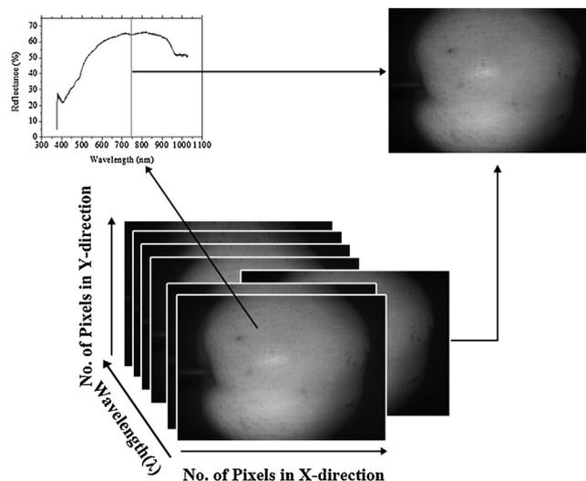
Fig. 2. Hyper spectral imaging.
