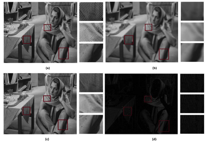
Fig. 2. Results of proposed method. (a) Original input image, (b) smoothed image after applying Gaussian filter ( \sigma = 5 ), (c) resultant structure part by proposed method and (d) texture part removed from the original image using proposed method.
