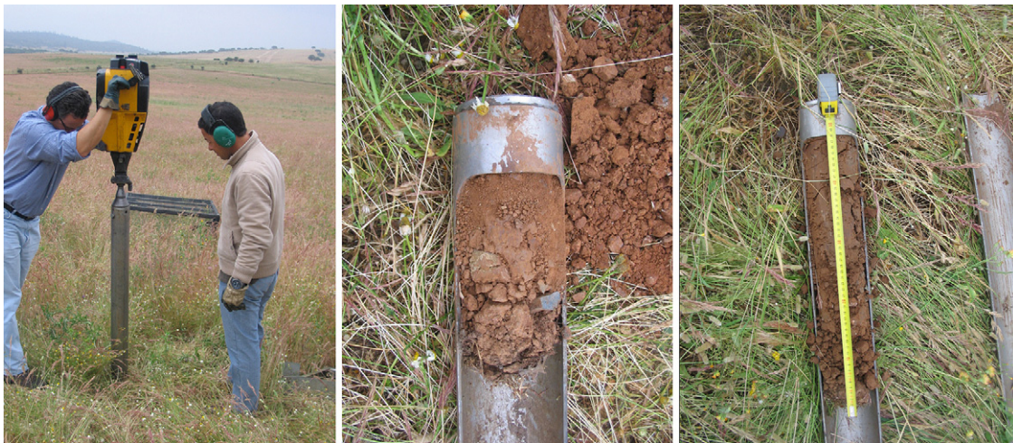
Fig. 1. Determination of soil profile (left) in top hills (centre) and bottom valley (right) in the experimental field.
