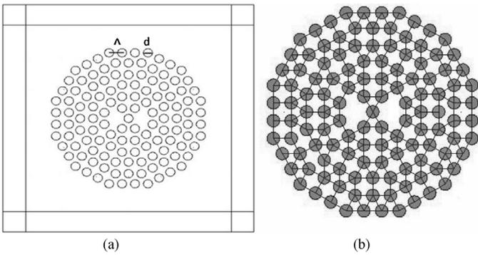
Fig. 1. Cross-sectional view of dual core PQF for,  $\Lambda=2\ \mu\text{m}$ ,  $d=1.4\ \mu\text{m}$  (a) with PML (b) with square and triangular lattice.
