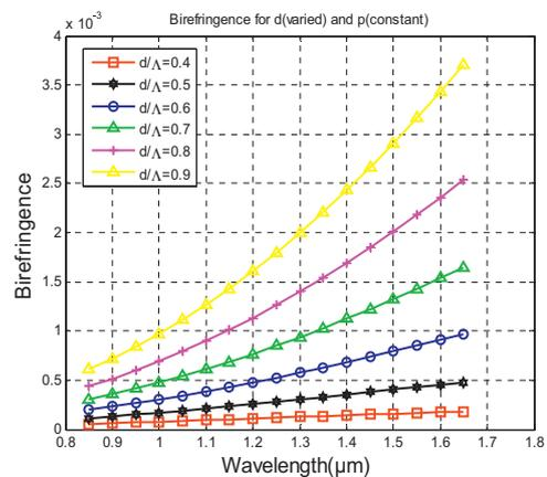
Fig. 4. Birefringence varying with wavelength for different  $d/\Lambda$  ratio.
