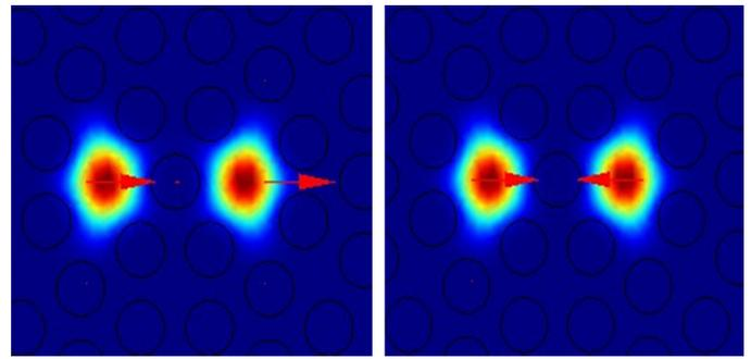
Fig. 3. Electric Field Intensity (a)  $x$ -polarized even mode (b)  $x$ -polarized odd mode.
