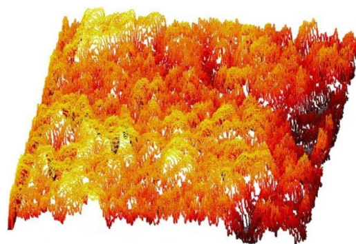
Fig. 2. Three-dimensional microscopic image surface profile scan of azo dye film.
